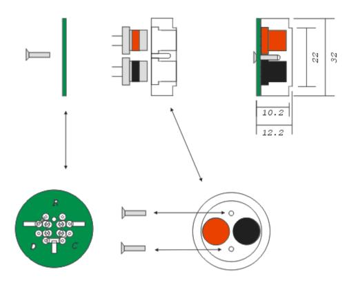
R—Reference D—Detector C—Compensator
